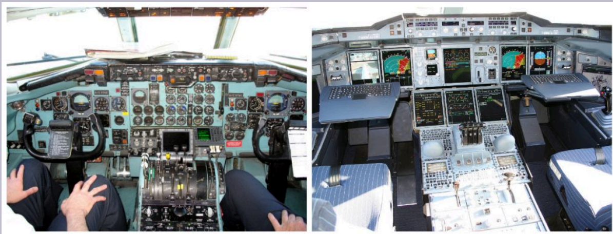
Figure 5.27. Initial design of the airplane cockpit (left); the digital design of the airplane cockpit (right), which has taken human factors into account.
